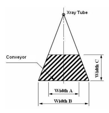
We select the type and type of X-Ray scanner accordingly with customer requirements. Product dimension must be included in the detection cone according to the table below.
