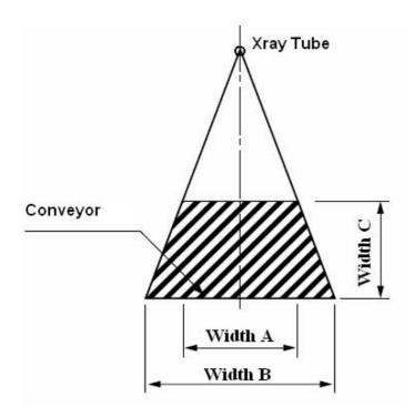
We select the type and type of X-Ray scanner accordingly with customer requirements. Product dimension must be included in the detection cone according to the table below.
