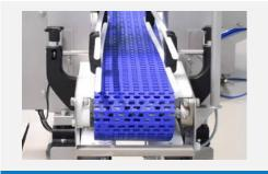
Modular tape used for difficult work conditions. Quick disassembly and possibility of easy washing of the tape makes it easy to keep the device in purity.
