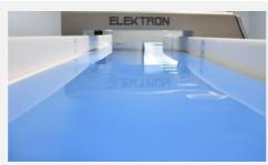
Polyurethane tape is used for transport of loose products or unpackaged products.
