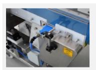
Blower recoil system for lightweight products up to 0.5 kg
